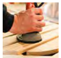
Edges are smoothed & rounded to eliminate splinters
